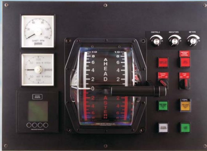
Bridge Control Station
